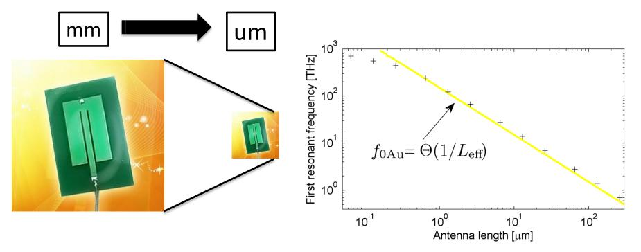
Ownscaling a traditional antenna to a few μm is not possible
