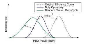
Fig. 5. Contribution of the duty cycle and random phase to the eventual efficiency curve. The duty cycle shifts the efficiency curve to lower values of energy by  $-10\log D$  dB. The random phase equalizes the curve, thus broadening the range of admissible input powers.
