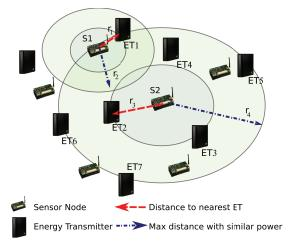
Fig. 1. Example of a WSN powered by wireless RF energy transfer. The number of coinciding RF waves generated by ETs with similar magnitude depends on the distance from the sensor to the closest ET. Larger distances imply more coinciding sources.
