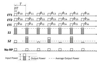
Fig. 3. DRAMA scheme. Each ET propagates RF waves with random phases  $\phi_{ik}$  in a duty-cycled manner with period T and duty cycle D.
