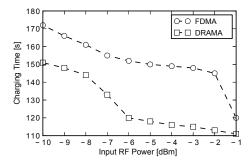
Fig. 9. Comparison of the charging times as a function the input power for DRAMA and FDMA.
