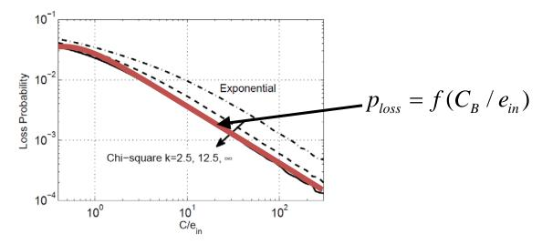
Therefore, the battery capacity CB can be estimated as:
