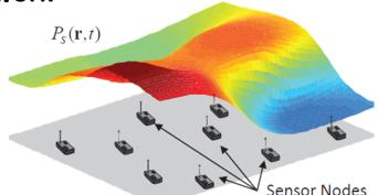
• We introduce the **Energy Field** as the average harvesting energy at a given position  ${\bf r}$  and a time t.
